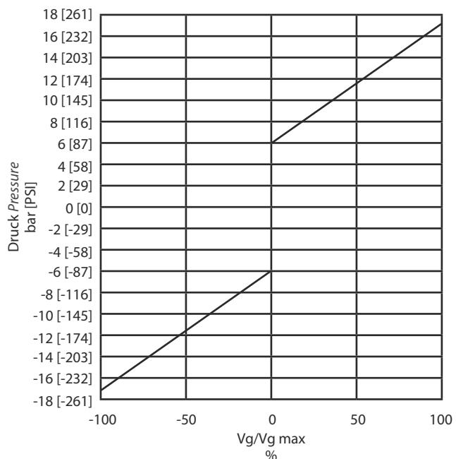
Pilot pressure: 6÷16 bar [87÷232 PSI] at ports a and b
