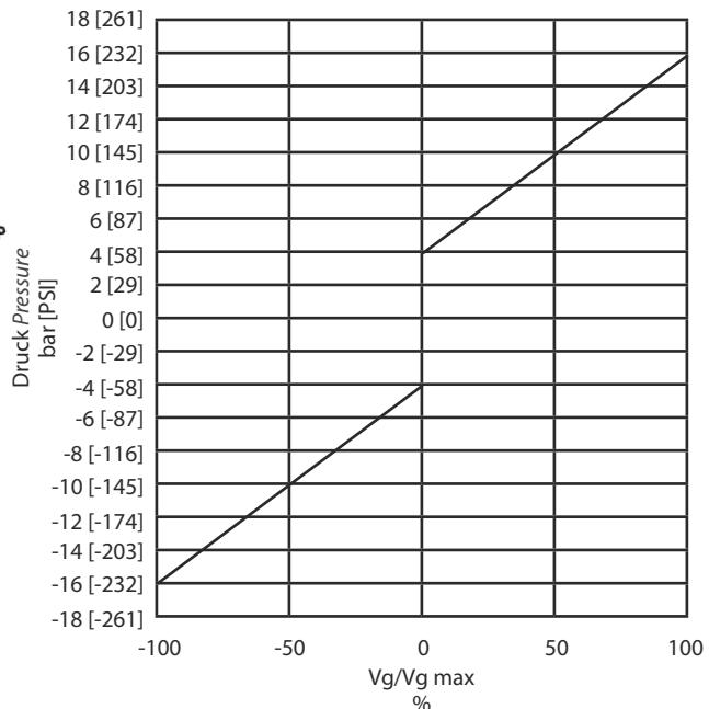
Pilot pressure: 4÷16 bar [58÷232 PSI] at ports a and b
