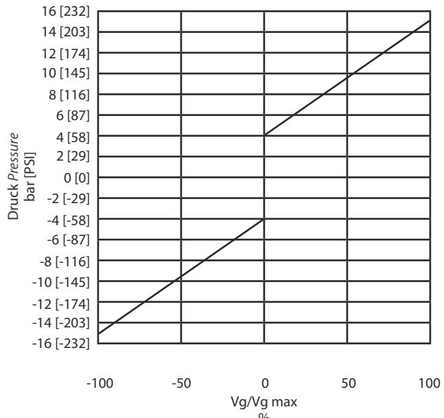
Pilot pressure: 6÷16 bar [87÷232 PSI] at ports a and b
